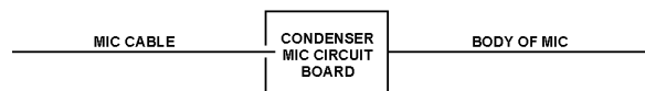
Figure 18 – The body of a microphone can be the other half of a dipole
