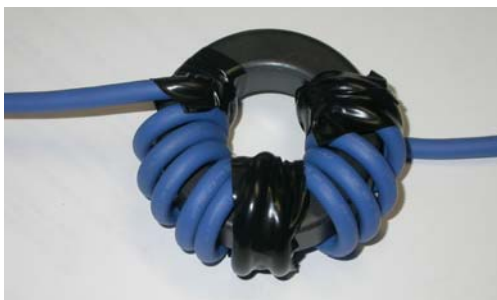
Figure 2 – A Multi-turn Choke on a 2.4" o.d. core
