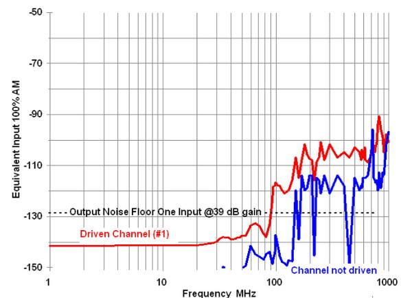
Figure 18 - Pin 1 susceptibility of the Sound Devices Mix Pre used for microphone testing. Pin 1 of channel 1 was driven and delegated to channel 1 out, channel 2 was delegated to channel 2 out, and both channels were set for 39 dB gain
