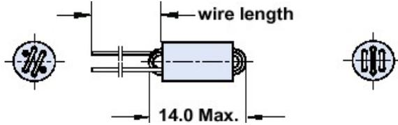
Figure 4 - The wound bead used in the isolators. Dimensions are mm
