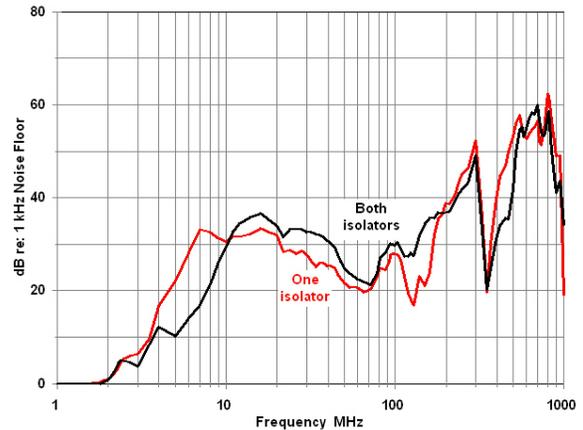
Figure 7 - Pin 1 susceptibility of mic TS-2-15 measured with the final test setup
