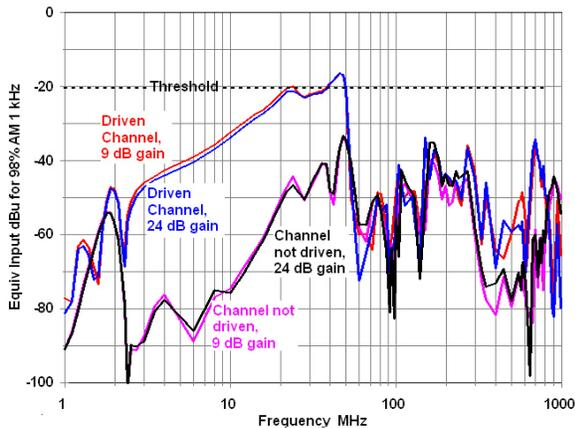
Figure 23 - Pin 1 susceptibility of a two-channel compressor/limiter from manufacturer #11. Pin 1 of only one channel is driven, and gains are equal.
