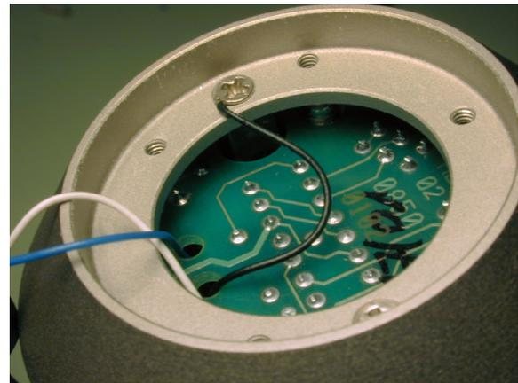
Figure 17 - New location for the black wire that was connected to pin 1 in microphone DL1-2-10
