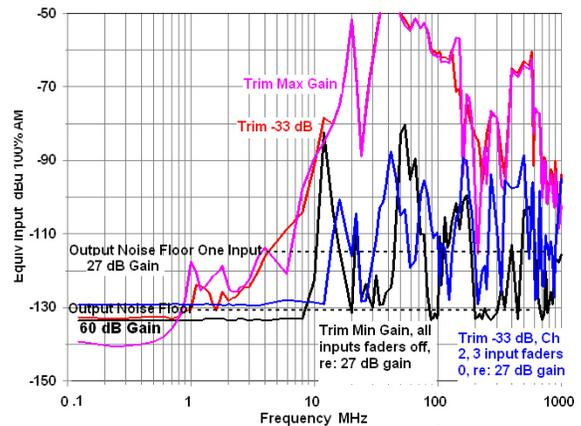
Figure 20 - Pin 1 susceptibility of 16-input mixer from manufacturer #10. Only pin 1 of channel 1 is driven for all tests.
