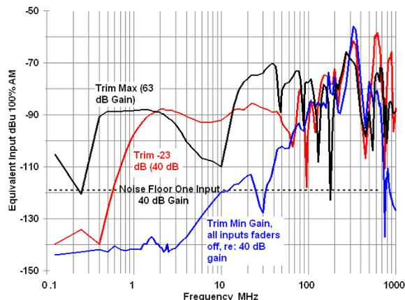
Figure 19 - Pin 1 susceptibility of 4-input mixer from manufacturer #10. Only pin 1 of channel 1 was driven for all tests.
