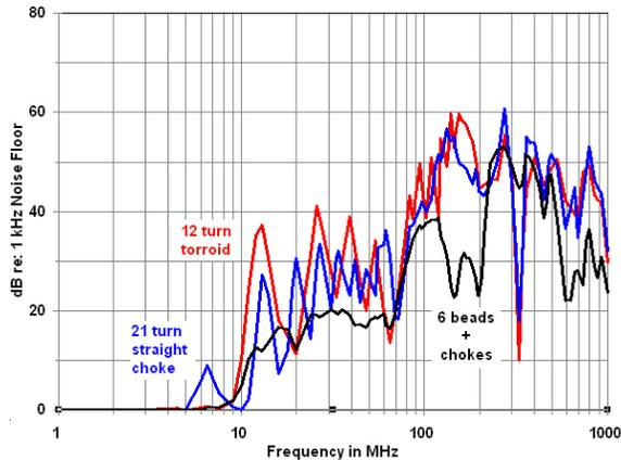
Figure 6 - Pin 1 susceptibility of mic TS-2-15 measured with early test setups
