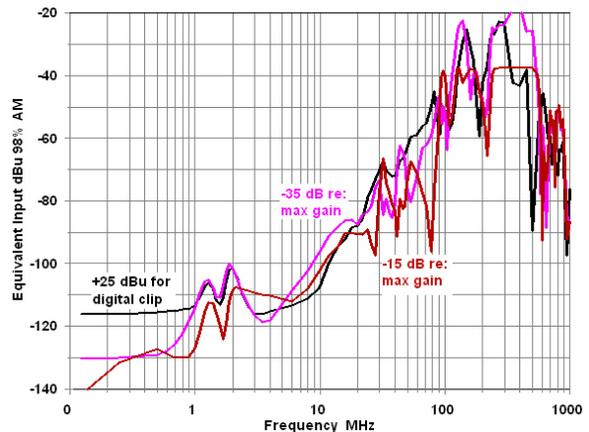
Figure 25 - Pin 1 susceptibility of the same portable DAT recorder for the driven channel expressed as equivalent input noise. The flat-topping of the highest gain curve is the input stage clipping.
