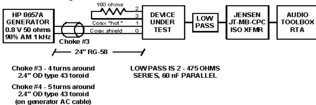
**Note: For a DUT where the XLR shells do not make contact or where the shell does not contact the chassis, the generator shield was connected to the chassis by the best convenient means.**
