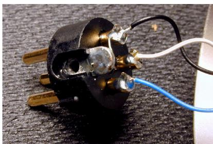
Figure 16 - Pin 1 termination in DL1-2-10 as manufactured
