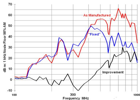
Figure 15- Result of moving one wire on microphone DL1-2-10
