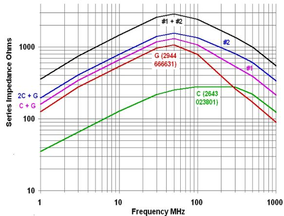
Figure 8 - Impedance of type C and G beads, individually and in various combinations
