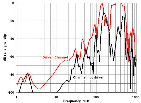
Figure 24 - Pin 1 susceptibility of a portable DAT recorder from manufacturer #12. Pin 1 of channel two is driven, gains of both channels are set for mic level at 35 dB below their maximum. At this gain setting, the input stage clips at -15 dBu and digital clip (to tape) is reached at -19 dBu..
