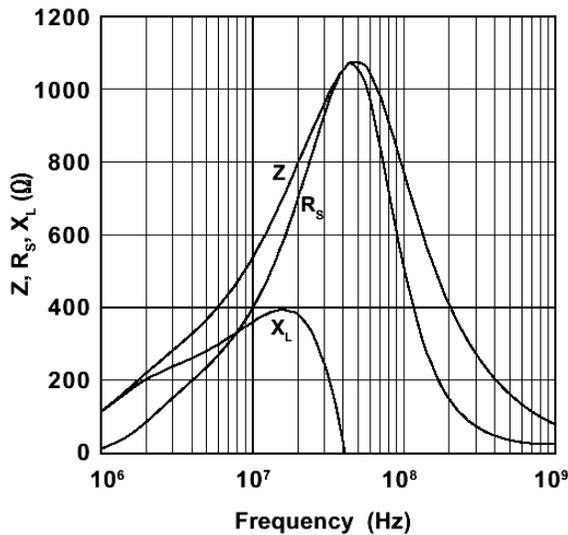
Figure 5 - Impedance of the multi-turn bead used in the isolators, identified as type G in Figure 2.
