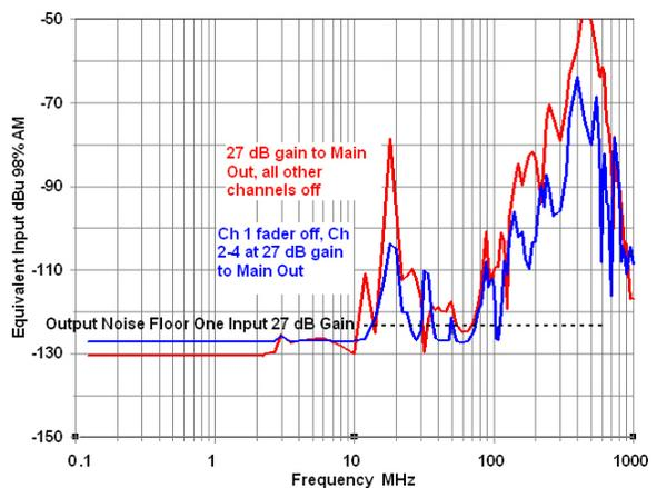
Figure 21 - Pin 1 susceptibility of a newer 4-input mixer from manufacturer #10. Only pin 1 of channel 1 is driven for all tests.
