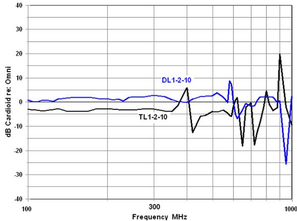
Figure 14 - Difference in Pin 1 susceptibility between omni and cardioid patterns of two switchable pattern microphones
