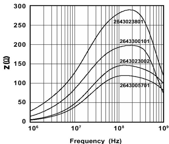
Figure 3 - Impedance of four beads of varying size and shape using type 43 material. The upper curve is for the largest of the group, which is the type C bead used in the isolators.
