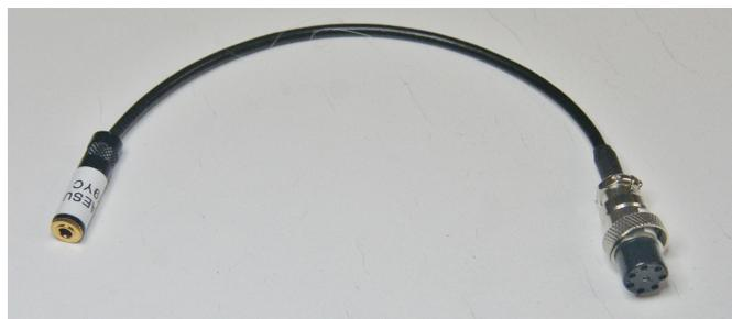
Fig 3 – Adapter For Computer Mic to Yaesu FT1000MP
