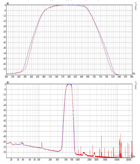
Driving the K3 with more noise made the greatest difference in the plateau effect noted in earlier measurements. The curves below is the response with the K3 IF set for 1kHz and with the 250Hz roofing filter or the 400 Hz roofing filter in place. The plateau of the response that was at about -25dB in earlier measurements is now at about -60dB. *The plateau was, indeed, an artifact of my measurement technique. – I simply wasn't driving the K3 with enough RF noise voltage.*
