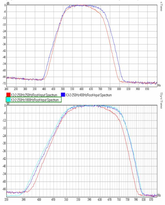
Again, data on this page is earlier, flawed data. The curve below is the response with the K3 IF set for 1kHz and with the 250Hz roofing filter in place. The plateau of the response at about -25dB is the result of not driving the signal chain with enough broadband noise voltage.
