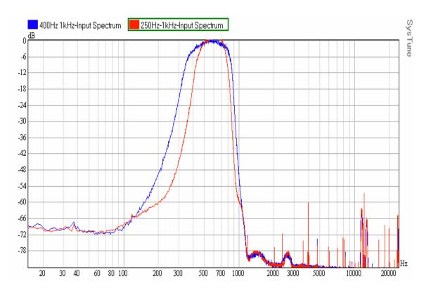
What follows is the original data set, with the K3 driven by insufficient noise voltage. Note that this data is from a different K3, which has different filters of the same type. Data on this page is for 250 Hz IF bandwidth with 250 Hz or 400 Hz roofing filters in place.
