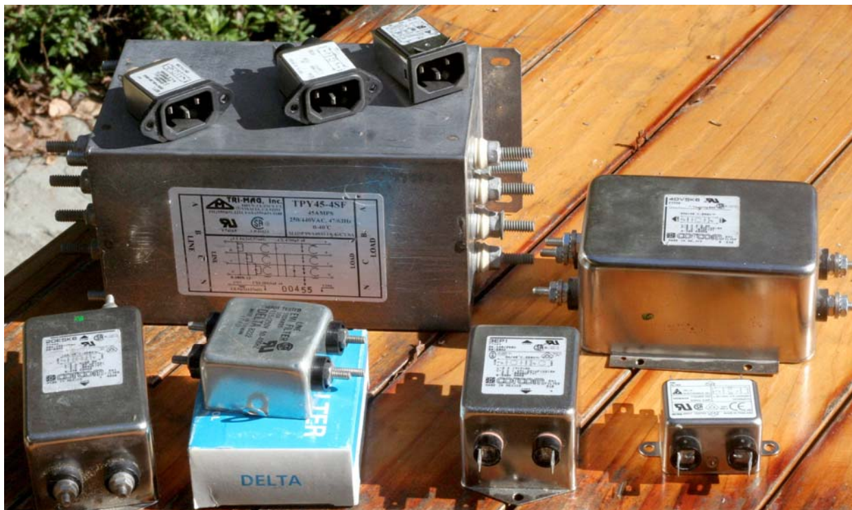
A selection of filters. The largest is a TriMag TPY45-4SF. Next largest (top right) is a Corcom 40VSK6. Bottom row, left to right: Corcom 20ESK6, Delta 10DKA5, Corcom 3EP1, Delta 10DBAG5. The small filters with IEC jacks are Corcom 6EF1, 6EH4, and a discontinued Delta product.
