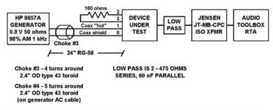
Note: For a DUT where the XLR shells do not make contact or where the shell does not contact the chassis, the generator shield was connected to the chassis by the best convenient means.
