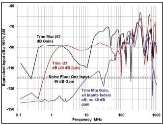
Figure 4 - The pin 1 problem in a small mix console known for picking up AM radio stations
