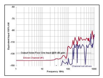
Figure 3 - The pin 1 test for a very good product
