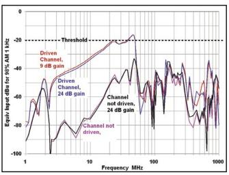
Figure 6 - A dual compressor/limiter with a serious pin 1 problem
