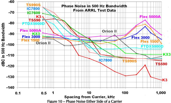
Figure 10 shows noise in a 500 Hz bandwidth, computed from the data by adding 10 log BW, which for 500 Hz is 27 dB. Not all plots show all radios – as I've added radios to the data set, I've omitted a few of the radios from each plot in the interest of clarity. In the 500 Hz plot, I've included all three Flex radios that ARRL has measured, which filled up the graph, so I omitted the Ten Tec Eagle and the IC7100. The relative performance does not change between the two plots.
