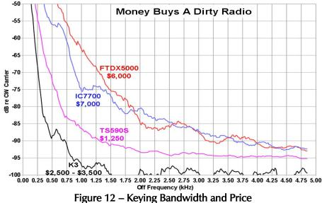
to much more expensive lcoms. The older Flex rigs have acceptable keying spectra, but phase noise is atrocious. Much is expected of the new Flex 6000 series; data provided by Flex looks very good, and ARRL Lab tests are eagerly awaited.
