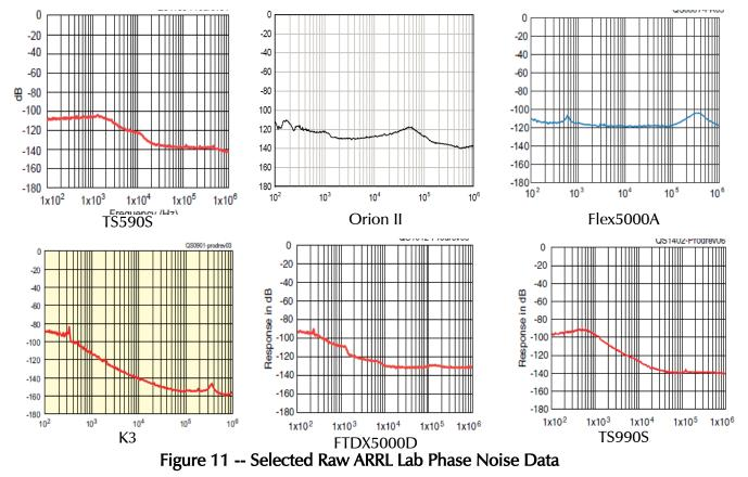
How Does This Correspond to What We Hear? The data presented here documents RF trash produced by the transceiver. A power amplifier will add its own noise and IMD to the transmitted signal, depending on how it is designed and operated. These issues are addressed in the K6XX talk previously referenced. What we hear can also be strongly affected by the ability of our receivers to handle strong signals, as well as the phase noise in our own receivers.
