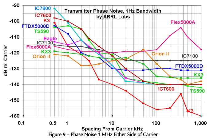
Figure 9 shows the full extent of the published ARRL data, to 1 MHz, for noise in a 1 Hz bandwidth, and the frequency axis is logarithmic. Several rigs have been added to this plot and the one that follows. This plot is useful in predicting which rigs create the least QRM when used at a multi-transmitter site like Field Day, a multi-op contesting station, or on a DXpedition. Wideband noise is also important to VHF + operators using the radio as a transverter base for weak signal work.
