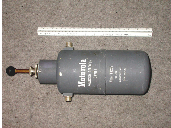
Fig 3 – A 450 MHz cavity and its response
