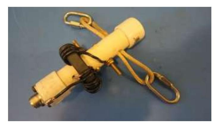
14 bifilar turns of #12 solid THHN on 2.4 inch type 31 ferrite core
