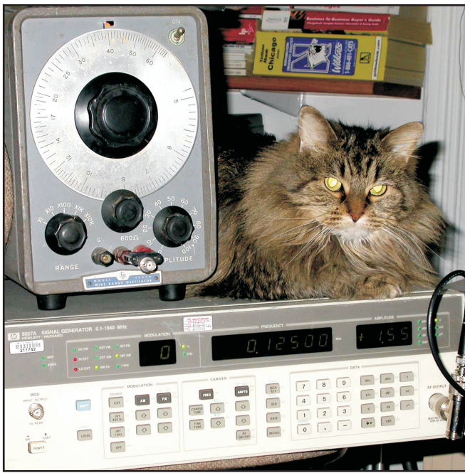
Fig. 2 - The HP 200CD audio generator was used for most data below 250 kHz; the HP 8657A at the higher frequencies.
